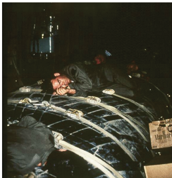
Fuel Bladders in C-130 Cargo Compartment
