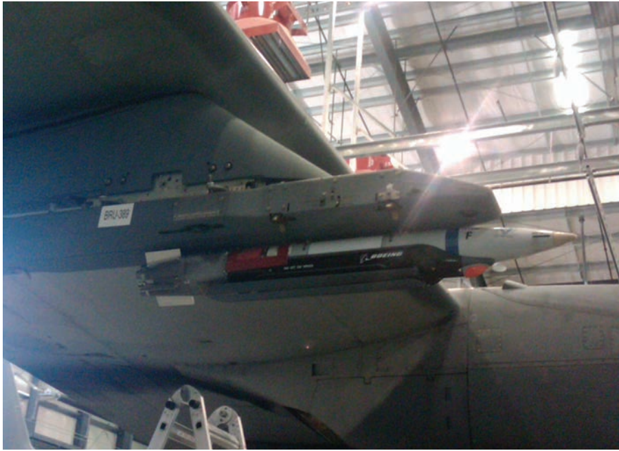
A GBU-39/B Small Diameter Bomb shown mounted under the right wing of an MC-130W.
