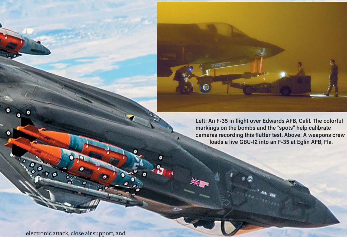
Left: An F-35 in flight over Edwards AFB, Calif. The colorful markings on the bombs and the "spots" help calibrate cameras recording this flutter test. Above: A weapons crew loads a live GBU-12 into an F-35 at Eglin AFB, Fla.
