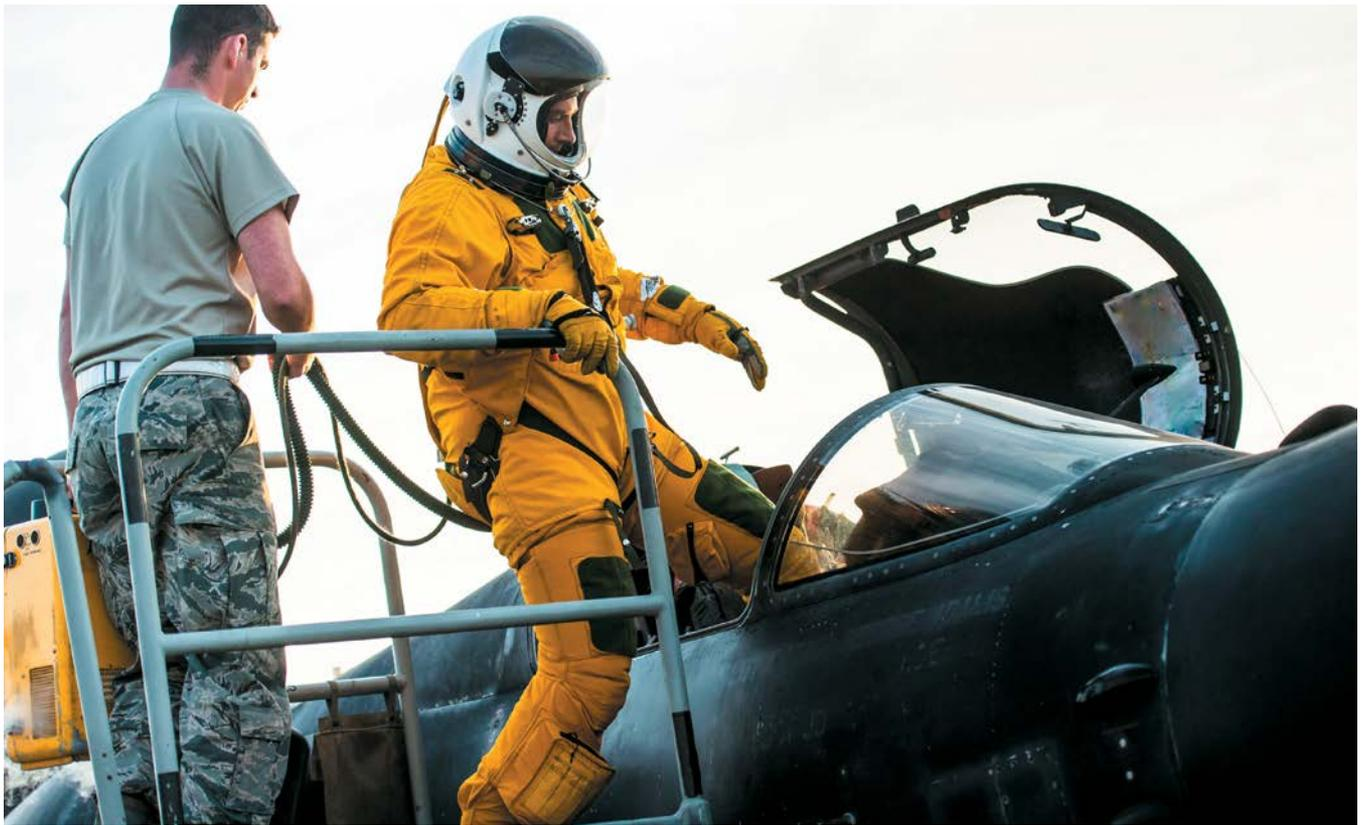
Maj. Ryan (last name withheld), a U-2 pilot, climbs into the cockpit for an Operation Inherent Resolve mission. U-2 pilots wear a pressurized space suit during flight to combat the effects of ultra-high altitude flight.
