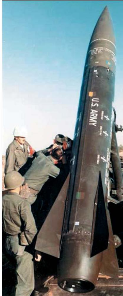
A Lance MGM-52C mobile surface-to-surface tactical missile, which could fire a one-kiloton atomic warhead up to 75 miles.
