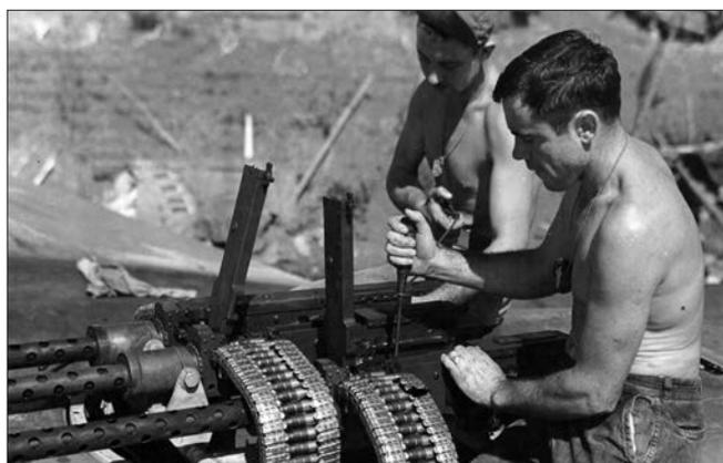
Airmen work on four .50 caliber machine guns in the upper turret of a P-61 night fighter on Saipan.
