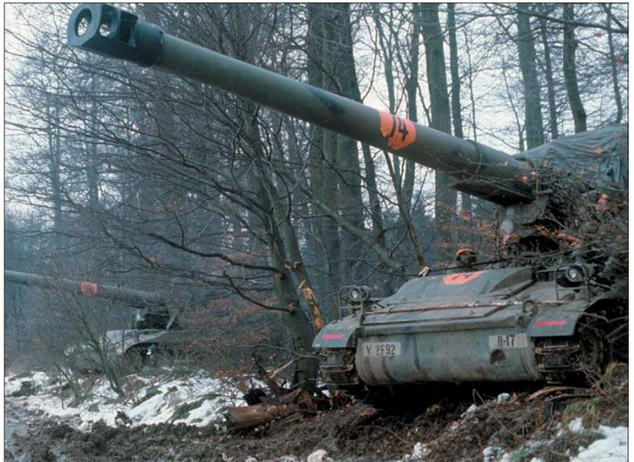
M110A2 203 mm self-propelled howitzers deployed along a line of trees during Exercise Reforger '85 near Weitershain, West Germany. The howitzers could fire atomic shells over 20 miles.
