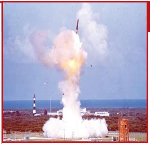
A Minuteman missile launches from Vandenberg AFB, Calif., in a periodic test of system reliability. The missiles were selected at random from those deployed in the field, pulled out of their silos, and brought to Vandenberg for testing.
