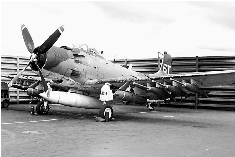
A-1H/J Sandy Sitting Alert (note the CBU canisters and fuze extenders or daisy cutters on the parent-mounted Mk-82s)
