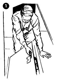
Lift the inflight inner escape door and rotate it to the vertical locked position.
