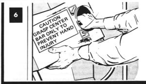
When door is in place, turn rotary locking handle onequarter turn counterclockwise to lock door.
