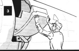
When door rotates and starts downward movement, support door and lower to extended position.
