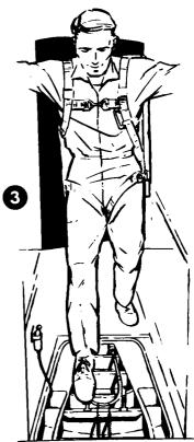
If pulling the D-handle fails to jettison the outer door, then the manual release pedal must be pushed to jettison the outer door.
