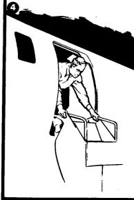
Grasp the handles and allow the door to rotate downward until door is in place, or it is resting on ground, depending on condition of airplane.
