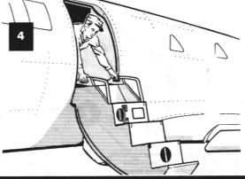
Raise door up and inward. The door will rotate and float inward.
