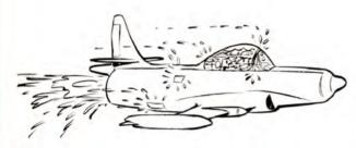
AS SOON AS THE FLAME-OUT IS EXPERIENCED, MOVE THE THROTTLE TO OFF TO PREVENT FLOODING THE ENGINE WITH FUEL.
