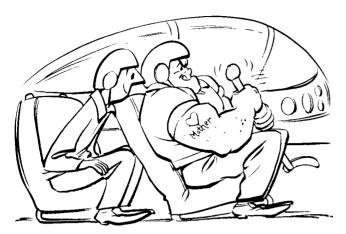
ON SOME AIRCRAFT THE AILERON BOOSTER IS OFF WHEN THE SHUT-OFF LEVER IS IN THE FORWARD POSITION. THE **ON** AND **OFF** POSITIONS ARE PLACARDED AND SHOULD ALWAYS BE VISUALLY CHECKED PRIOR TO MOVING THE LEVER TO ASSURE THAT HYDRAULIC BOOST WILL BE AVAILABLE FOR TAKE-OFF.
