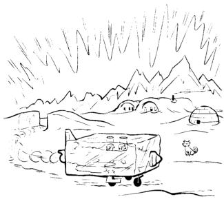
FAILURE TO REMOVE SNOW AND ICE ACCUMULATED ON AIRCRAFT WHILE ON THE GROUND CAN RESULT IN SERIOUS AERO-DYNAMIC AND STRUCTURAL EFFECTS WHEN FLIGHT IS ATTEMPTED.
