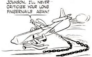
THE SPEED BRAKES MUST BE RETRACTED IN ORDER TO MAKE A SUCCESSFUL BARRIER ENGAGEMENT. IF THE SPEED BRAKES ARE EXTENDED, THEY WILL DEFLECT THE BARRIER ARRESTING CABLE DOWNWARD, CAUSING THE MAIN LANDING GEAR TO PASS OVER THE CABLE INSTEAD OF ENGAGING IT.
