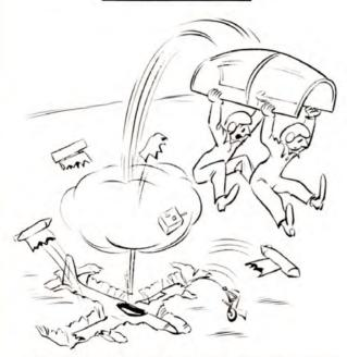
IN ANY GROUND SITUATION WHERE THERE IS A POSSIBILITY OF FUEL SPILLAGE IN THE VICINITY OF THE AIRCRAFT, THE CANOPY SHOULD NOT BE JETTISONED, EXCEPT AS A LAST RESORT, DUE TO THE ADDITIONAL FIRE HAZARD CREATED BY DETONATION OF THE CANOPY REMOVER CARTRIDGE.
