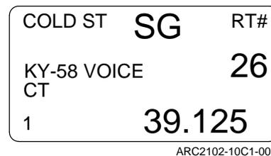
**Figure 1-123. SINCARS Cold Start RSC Screen**
