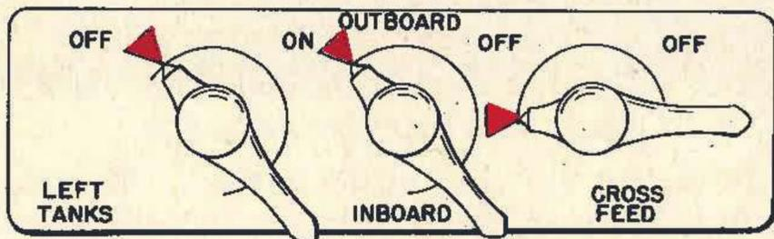
**To Operate Both Engines from Right Outboard Tank**
