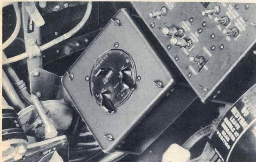
Figure 17 —Pilot's Ignition Switch Panel
