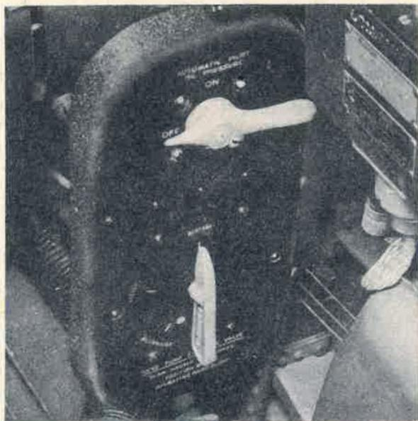
Figure 24 — Hydraulic Hand Pump Selector Valve
