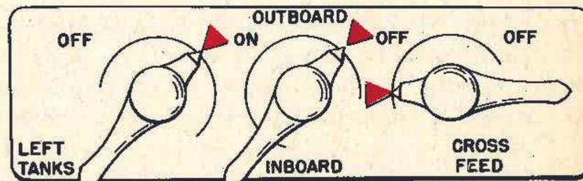
**To Operate Right-Hand Engine from Left Outboard Tank**
