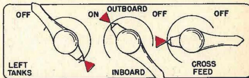
**To Transfer Fuel from Left Inboard to Right Outboard Tank**
