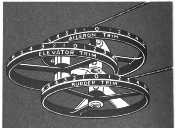
1. Set all trim tabs at neutral. To do this, move the 0 of each trim tab wheel into the line of vision between your eyes and the shaft on which the wheel is mounted.
