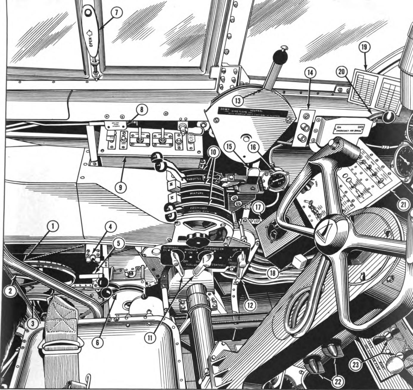
**Controls, Switches, Instruments (at Pilot's Left)**
