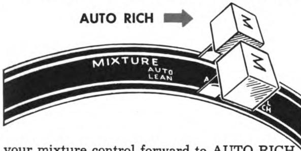
your mixture control forward to AUTO RICH and leave it there. If the engine does not start, be sure the starter jaws are disengaged before you energize the starter for another try. If your throttle has been opened 1/3 or more, pull it back quickly and smoothly as the engine picks up speed. This prevents backfiring.
