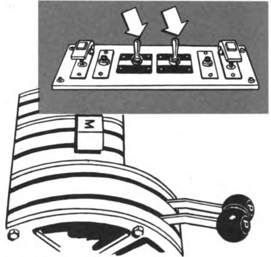
However, as you know, with the propellers at a fixed pitch, you must increase the engine rpm whenever you want to climb, and decrease it when you want to descend. To do this, hold the propeller selector switch either in the **DECREASE** or **INCREASE** position until the desired rpm is reached. Remember that the selector switch is spring-loaded. As soon as you let it go, it snaps back to the **FIXED PITCH** position.
