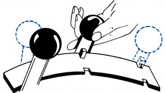
taking place, for the oil pressure drops and returns to a reading about 5 psi below its previous one. This reaction lags an instant or two behind the movement of the blower handle. At the same time, the manifold pressure tends to surge upward. Pull back the throttle to prevent it from exceeding the value you want to maintain temporarily. When the shift is completed, advance the throttle to the desired setting. Now, repeat the procedure with the other blower.
