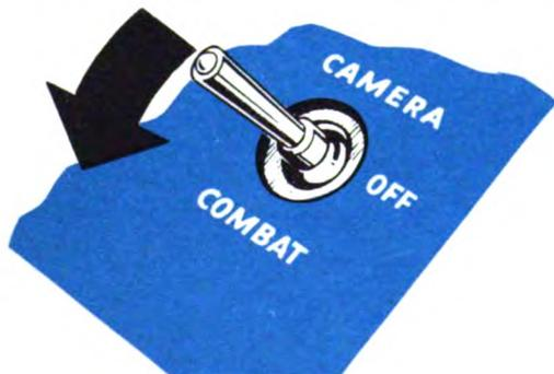
switch is in the OFF position it acts as a safety for all guns.) Adjust your gunsight to the desired brilliancy by turning the rheostat at the bottom of the electrical panel
