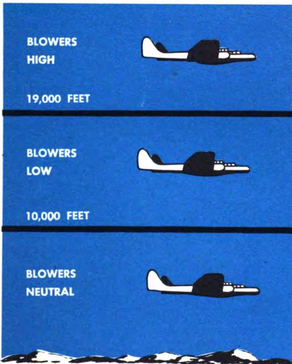
**Remember, the blowers steal horsepower from the propellers.** In LOW position, they use up about 200 Hp more than they do in NEUTRAL. In HIGH position, they use up approximately 350 Hp more than they do in NEUTRAL. Therefore, if you are going to climb to a height just under the point at which you normally would shift blowers, don't shift them, even when your manifold pressure seems a lit-
