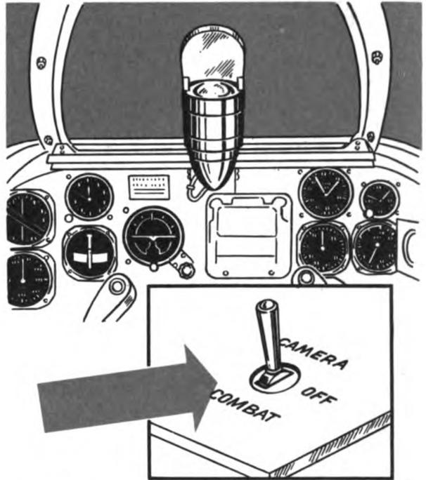
The P-61's pilot has an optical gunsight (100 mil), which is mounted directly in back of his bulletproof windshield and at the top of the instrument panel. With this sight, he aims the fixed guns and directs the fire of the movable guns when they are in the strafing position.
