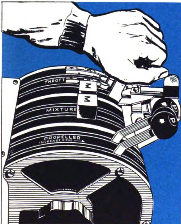
time leans out the fuel mixture. When you have pushed the throttles wide open, flip the lever to the left with your thumb. With the water injection feature in use, the water pressure gage at the right of your cockpit should now register 17 psi. If your water supply becomes exhausted, be sure to turn off the water injection system.
