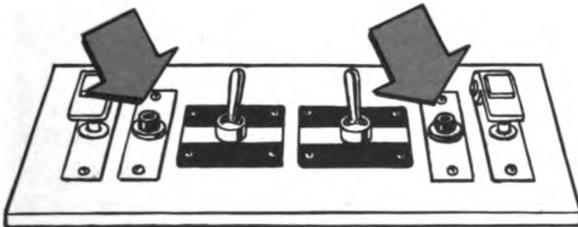
This type of circuit breaker is designed to carry extremely high loads when you hold the button in. By making careful use of this feature, you may set the propeller blades at a satisfactory angle in spite of a damaged or overloaded propeller circuit. **But don't hold the button in except in an emergency.**
