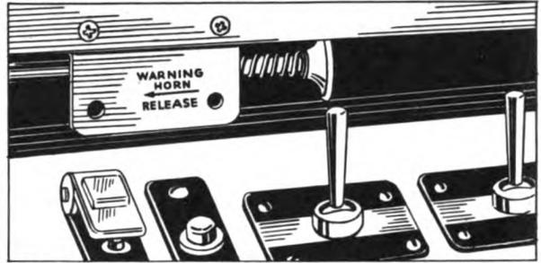
In addition to checking on the operation of the landing gear warning horn when you are about to land, also look at your landing gear indicator on the instrument panel. It should show that the wheels are down. In the daytime, take the added precaution of glancing out the window to check the position of each main wheel. Then, look at the front portion of either engine cowl. If these engine cowls are kept clean and shiny, they're as good as mirrors for telling you the position of the nosewheel.
