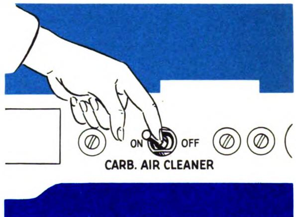
forces the air to flow through a cleaner. If, on the other hand, no dust is blowing, hold the filter switch in the **OFF** position for a few seconds to make certain the cleaner will not operate.
