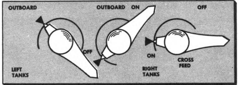
**How to Operate An Engine from An Opposite Tank**
