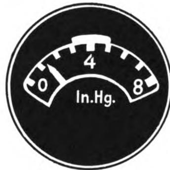
The automatic pilot's suction gage should read between 3.75" and 4.25" Hg. at all times.
