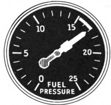
fuel booster pump and check to see that the engine-driven fuel pump is maintaining a pressure of 15-17 psi.
