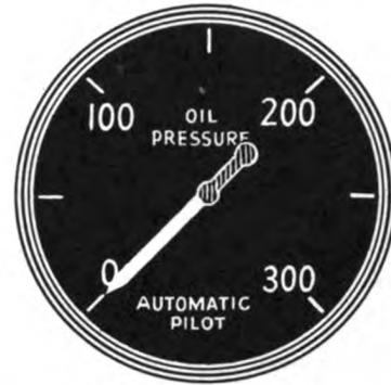
The automatic pilot oil pressure gage should read 100-125 psi for normal operation. Sometimes, it will read low before you engage the automatic pilot. Generally, however, it promptly registers a normal reading after the automatic pilot is engaged. If it does not, disengage the automatic pilot and enter your unhappy discovery on the Form 1.
