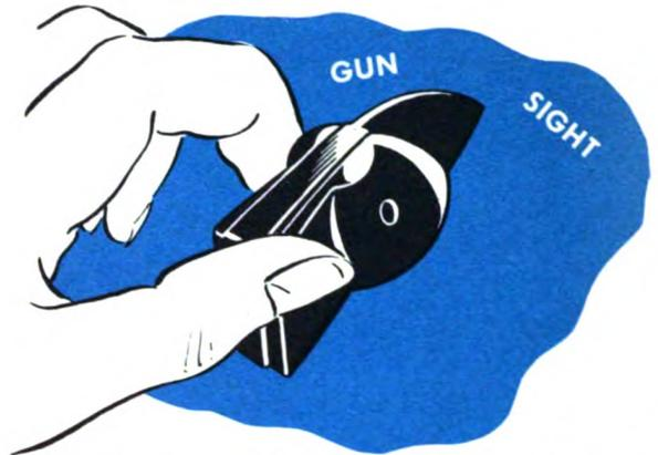
Fire the guns with the button (on top) and the trigger (underneath) at the righthand side
