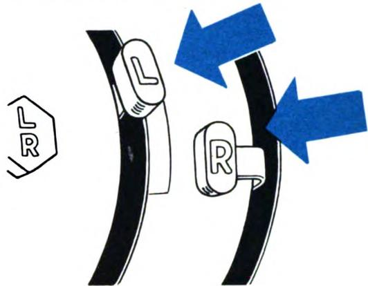
12. Be sure the oil pressure for your automatic pilot is **OFF**, and that the automatic pilot itself is not engaged.
