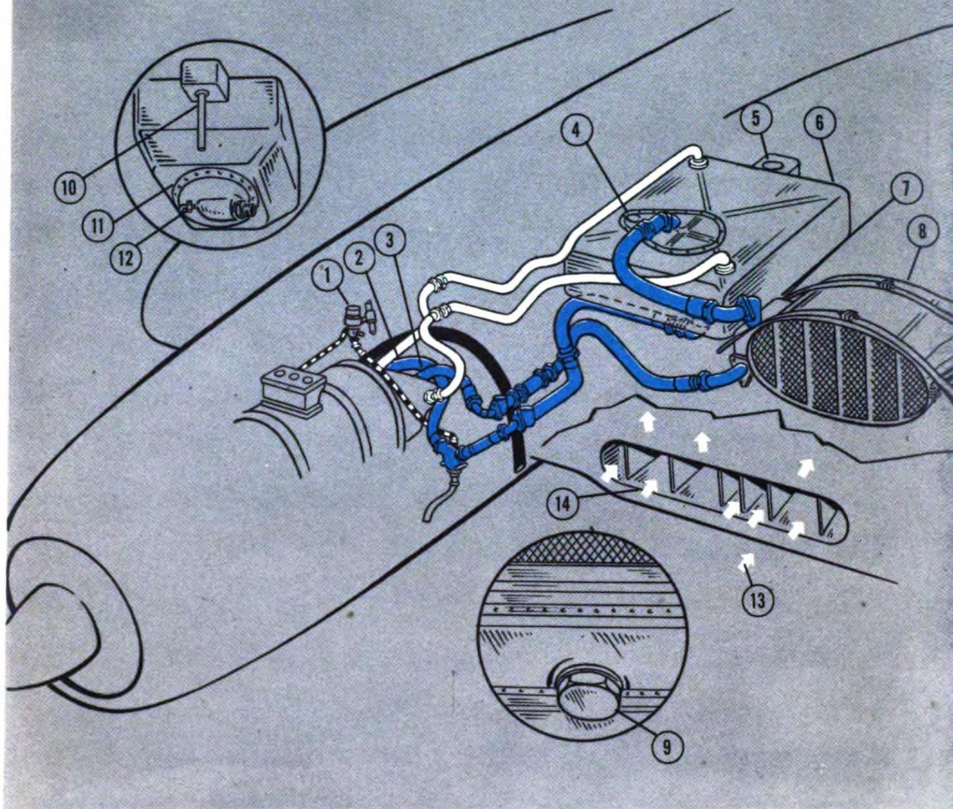
speed booster pump which you may use to supply fuel to the engine-driven pumps. Normally, the booster pumps are not used while the airplane is cruising, unless fuel pressure is low. The booster pumps operate either in LOW or HIGH position and, if the engine-driven pumps fail, you may use the boosters to supply fuel to
