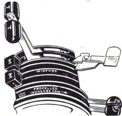
3. Be sure your mixture control is in IDLE CUT-OFF position. While the booster pump is ON, during starting procedure, the mixture control should never be out of the IDLE CUT-OFF position for more than a second or two. Otherwise, the induction system becomes flooded, creating a bad fire hazard.
