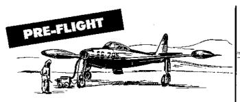
1. When the ambient temperature is 0°C (32°F) or lower, use a portable heater to blow hot air into the airplane air inlet duct for a period of 10-15 minutes. This procedure is necessary to prevent the starter-generator unit from being damaged due to ice seizure of the compressor rotor.
