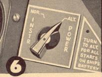
Instrument power switch ALT for ignition during airstart.
