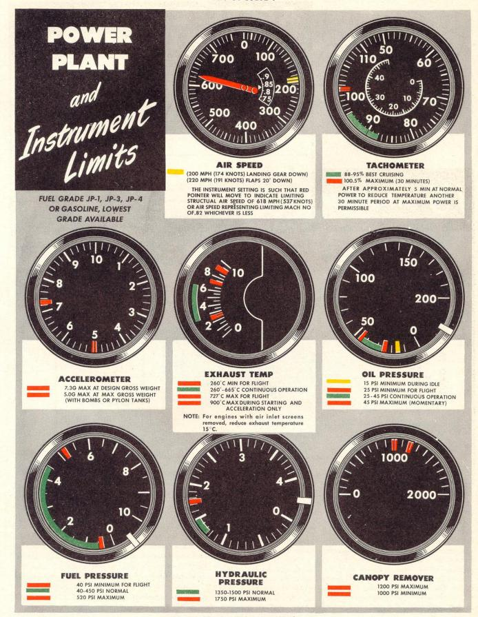
Figure 5-2. Instrument Markings
