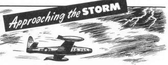
It is imperative that you prepare the airplane prior to entering a zone of turbulent air. If the storm cannot be seen, its proximity can be detected by radio crash static. Prepare the airplane as follows:
