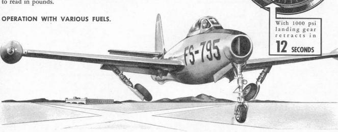
Figure 7-3. Landing Gear Retraction Time
