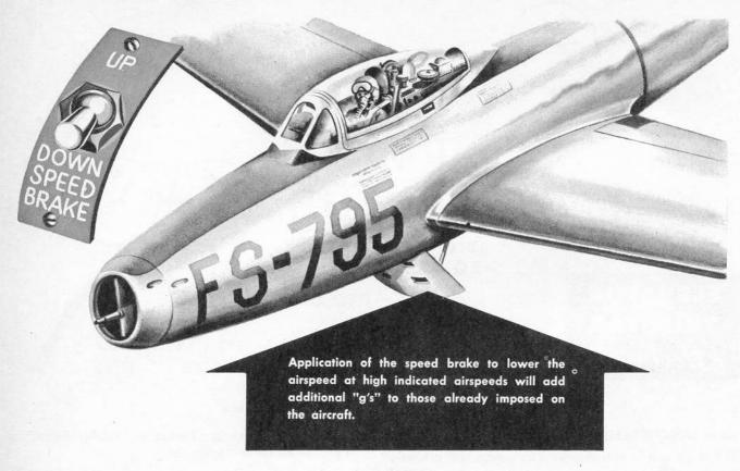
Figure 6-9. Speed Brake Effect
