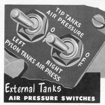
Figure 1-9. External Tanks Air Pressure Switches
