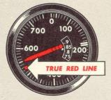
A good rule of thumb to remember is: Each "g" imposed on the airplane lowers the red-line speed (critical Mach number) by 5 mph. (Example: Red-line speed of 550 is reduced to 525 when 5 "g's" are imposed on airplane).
