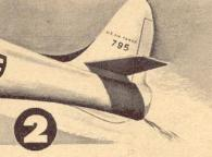
Raise nose to drain out unburned fuel through tail pipe.
