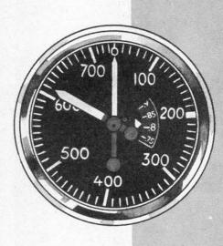
1. Do not exceed 260 mph IAS with flaps set at 20 degrees. The flaps will automatically retract from 40 to 20 degrees if the airspeed exceeds 220 mph IAS.
