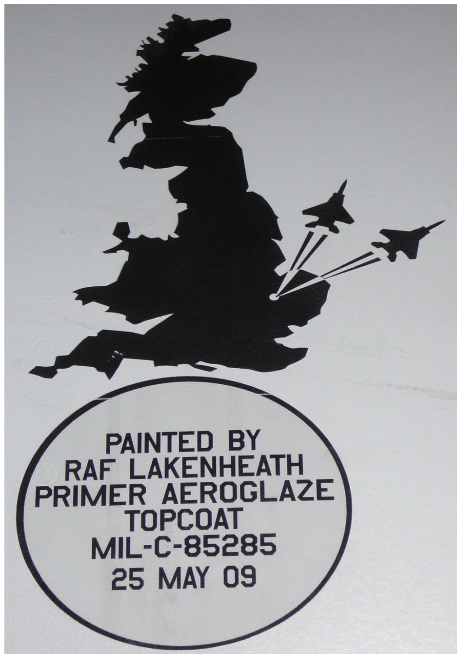
Figure A21.1. 48 FW Paint Identification Block.
