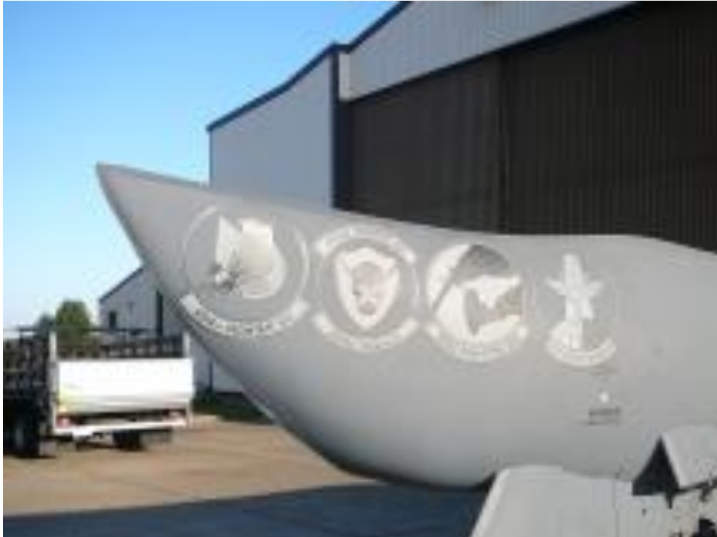
Figure A12.1. 48 FW Left CFT Paint Configuration for 48 FW & 48 OG Commanders' Aircraft.
