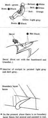
On this model cut off the boundary layer fence and paint it red.
