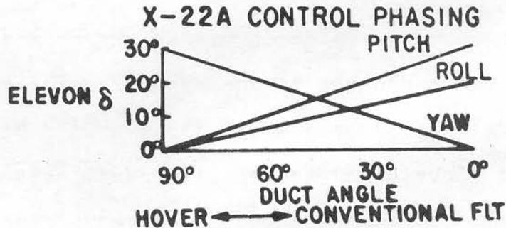
In conventional flight the elevons provide roll and pitch control in the conventional manner. The handling characteristics are very good with slight adverse yaw which builds up as the turn develops making it necessary to hold rudder into the turn. The yaw spring is turned on during transition and conventional flight to provide a conventional rudder force gradient. For hovering flight the yaw spring should be disengaged which provides very good rudder forces for directional control.
