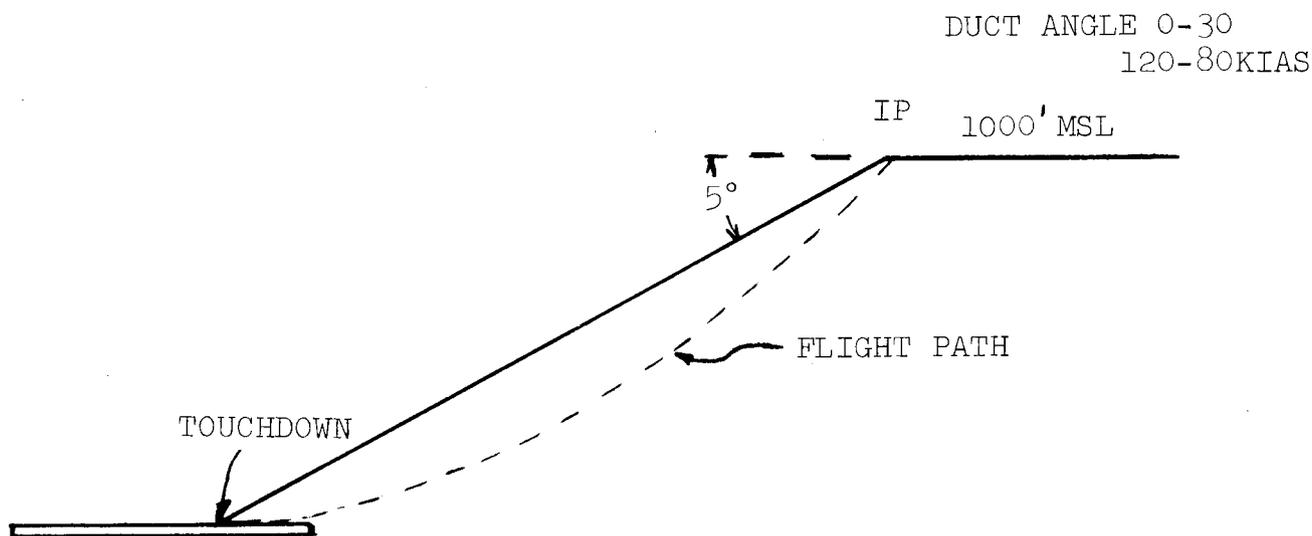
6. When firmly on the runway, reduce power and rotate ducts upward to reduce speed.
