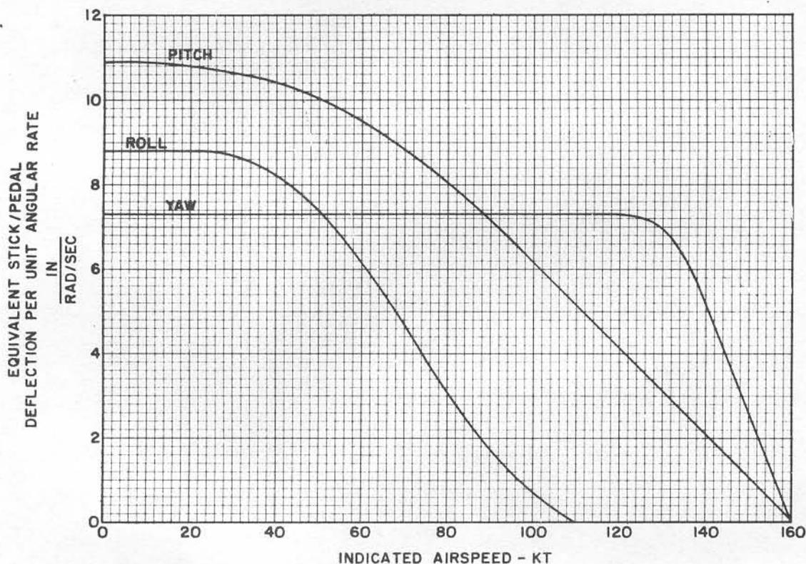
At speeds above 160 knots the system is completely phased out as aerodynamic damping provides adequate stability at higher airspeeds. The SAS is fully duplicated, and operation on one system results in reduced rate damping and authority, degrading the handling characteristics very little. The aircraft can also be flown in all flight conditions without undue difficulty with SAS-off. The most difficult flight conditions without SAS is in the final stages
